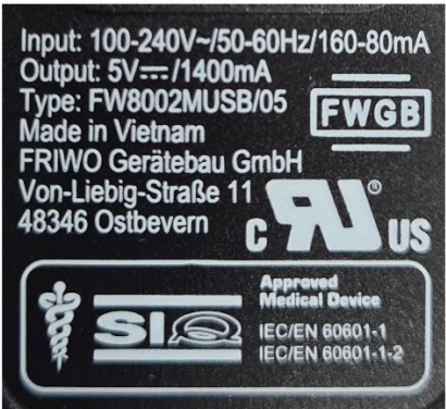
Fig. 13 - Mains power supply data plate
